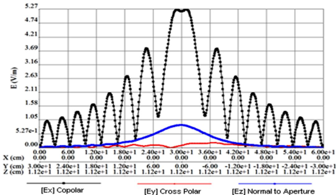
Fig. 6 Feed lowered by 2cm: E-Field variation along Line CD on the Aperture plane.
