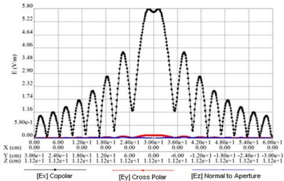
Fig. 3 Feed at Focal: E-Field variation along Line CD on the Aperture plane.
