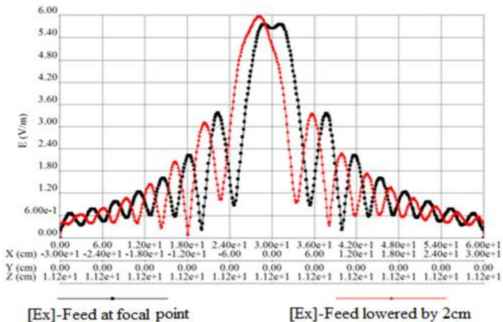
Fig. 8 Copolar component on the Aperture plane along Line AB
