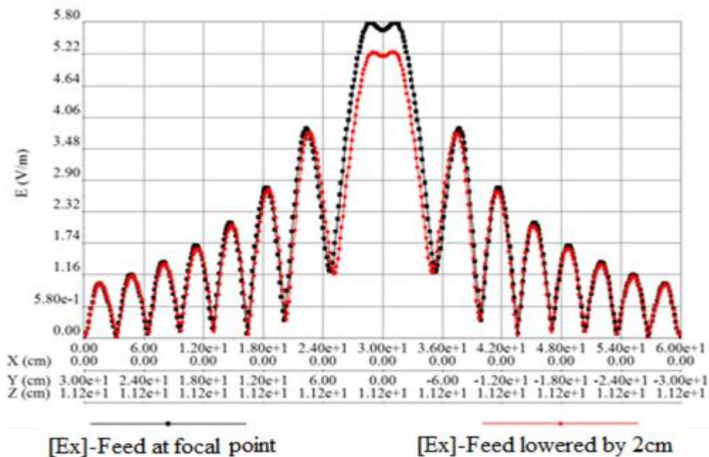
Fig. 9 Copolar Component on the Aperture plane along Line CD
