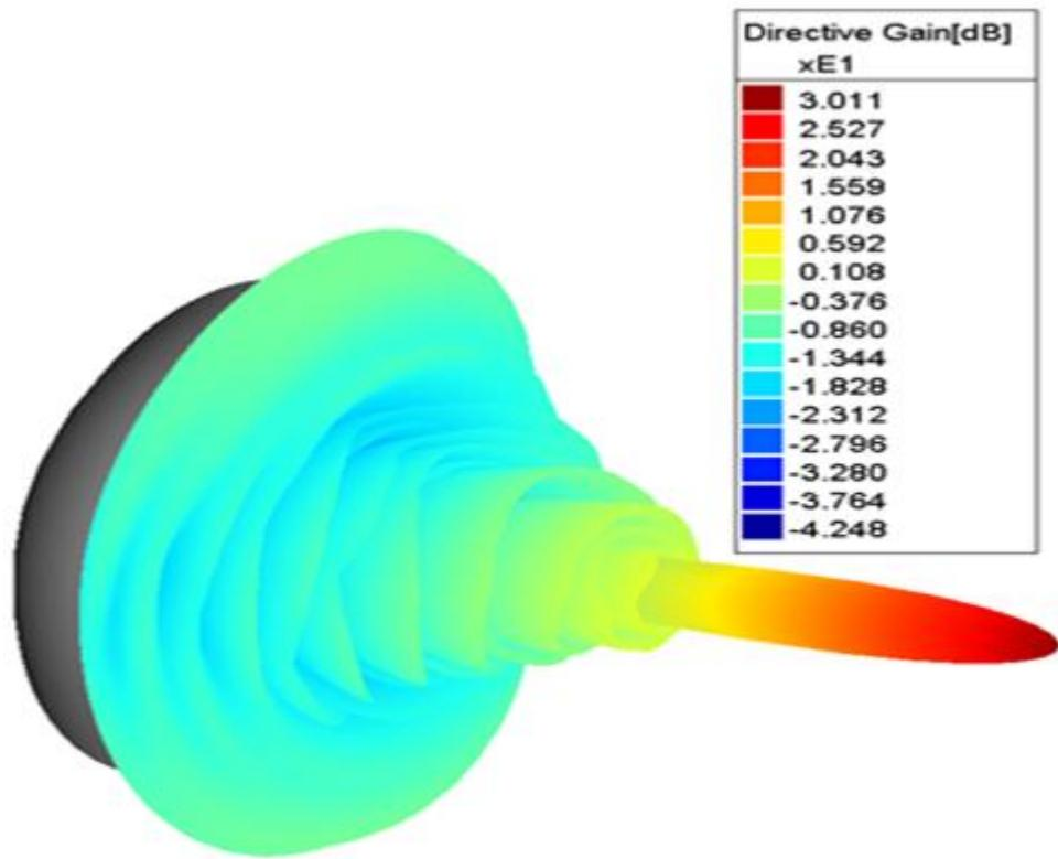
Fig. 7 Feed lowered by 2cm
