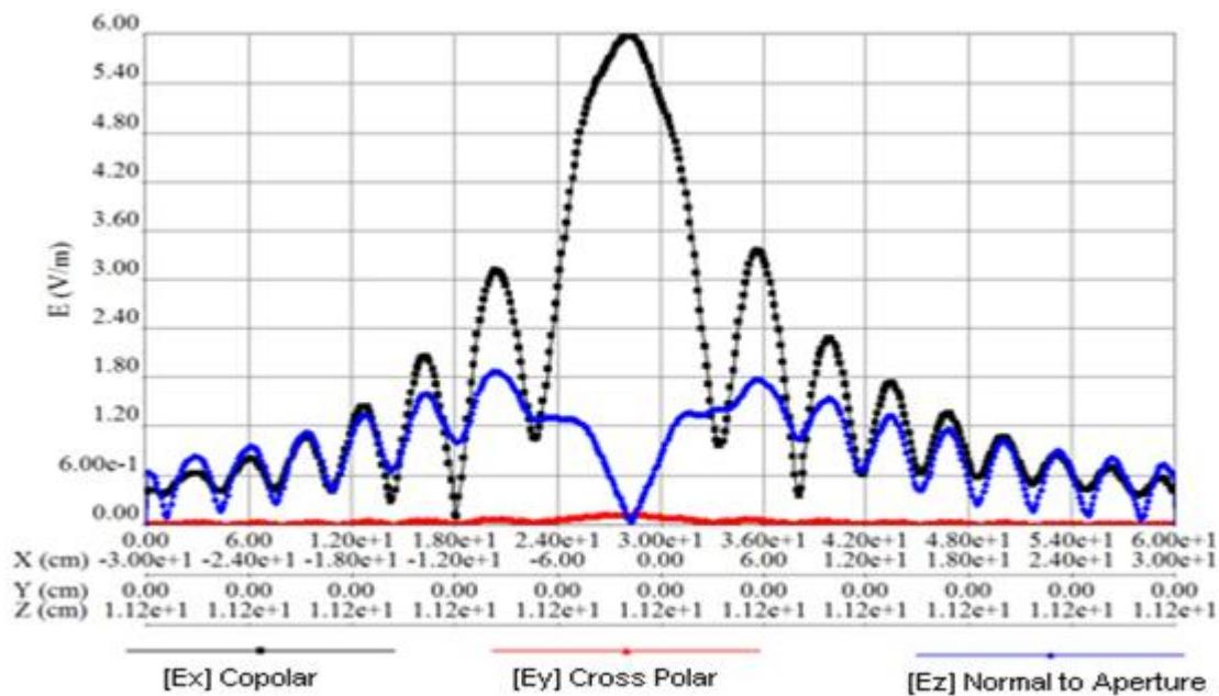
Fig. 5 Feed lowered by 2cm: E-field variation along line AB on the aperture plane.
