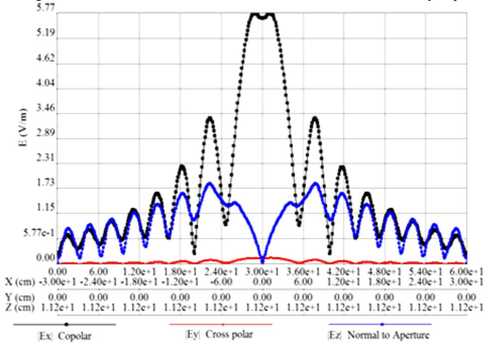
Fig. 2 Feed at Focus: E-Field variation along Line AB on the aperture plane.
