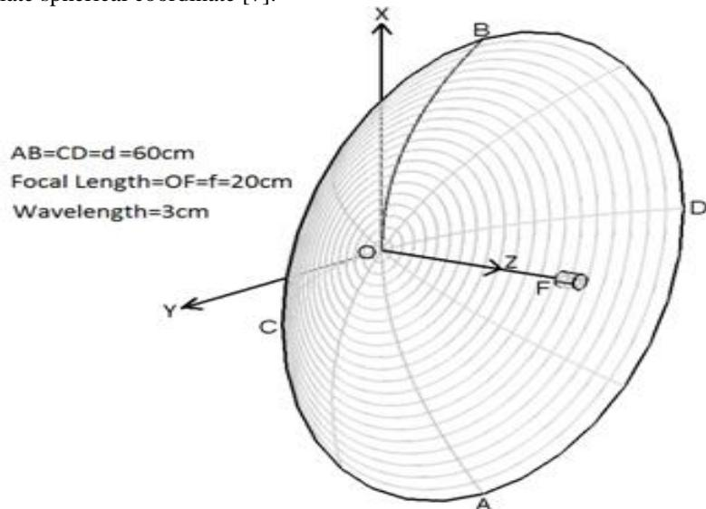
Fig. 1 Paraboloidal reflector designed for focal length of 20cm and wavelength of 3cm.
