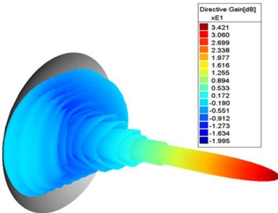
Fig. 4 Directive gain of prime focus paraboloid aperture diameter=60cm, Focal length=20cm Frequency of operation=10GHz.
